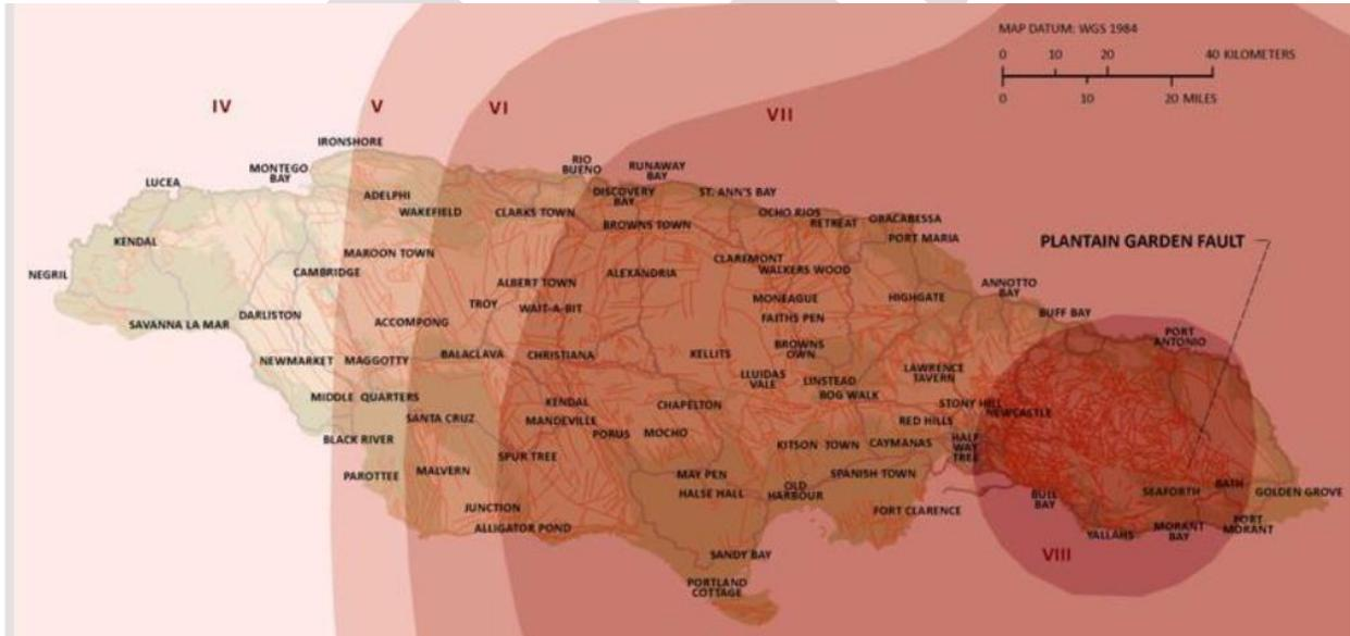
Figure 6.2: 100-year Return Period Earthquake of Magnitude VIII from within the Blue Mountains Block (Mona GeolInformatics and UWI Earthquake Unit, unknown)
