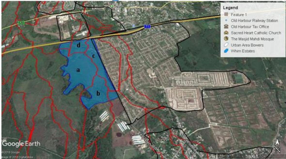
Figure 5.9: Catchment and Drainage Network showing downstream Flow towards the Whim Estates
